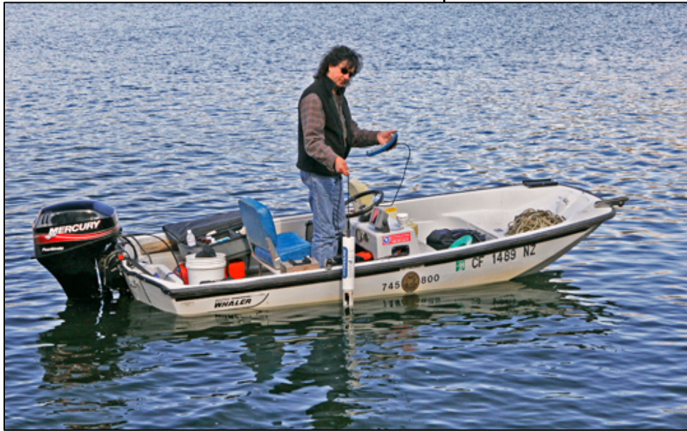
San Francisco Public Utilities Commission limnologist Mike Horvath uses sophisticated equipment to locate the thermocline of a stratified reservoir, but you can find it by setting the sensitivity of your depth finder to high.
